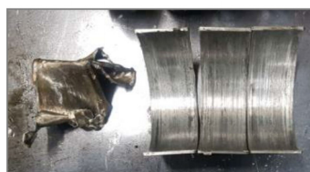
< Connecting rod bearing seizure >
